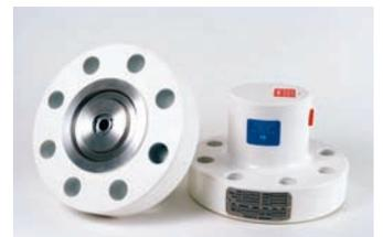
Porting through the spools has a through-bore equivalent to 1/2" and 1" cross-section areas respectively. The spool-to-body primary seal is metal-to-metal, with a PTFE secondary seal.
