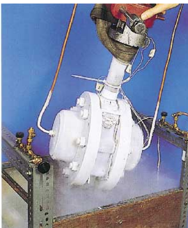
Solent & Pratt valve undergoing cryogenic testing at Southampton University.
